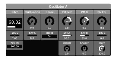
The two sine wave oscillators are the only signal sources. With a random frequency fluctuation they can also produce tunable noise. They are equipped with three phase modulation inputs for:
