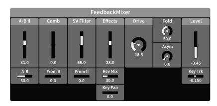
This mixer combines the following signals for the feedback bus: the outputs of the Comb Filter and the State Variable Filter and the output of the Effects chain, with a separately adjustable amount of Reverb. It includes a sine shaper for the sum signal.
