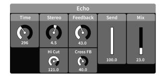
A stereo delay effect with adjustable cross-feedback.
