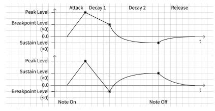
Envelope C - "Retrigger Hardness" Parameter (in monophonic mode):
