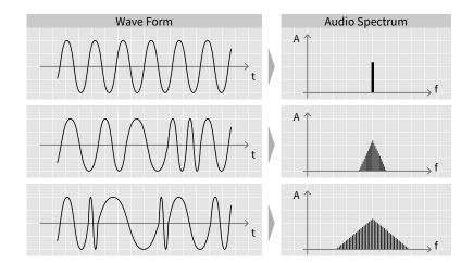
Oscillator signal with self modulation and different amounts of fluctuation:
