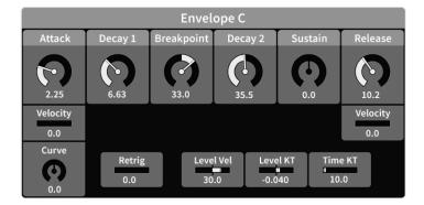
The third ADBDSR envelope has bipolar Breakpoint and Sustain levels. It can modulate:
